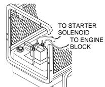
Figure 15 - Connecting Positive and Negative Cables to Battery (Model RGH11000AIE Shown)
